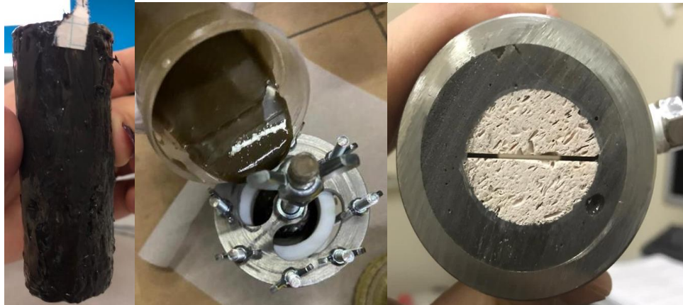
Fig. 17. Core preparation process before the experiment
