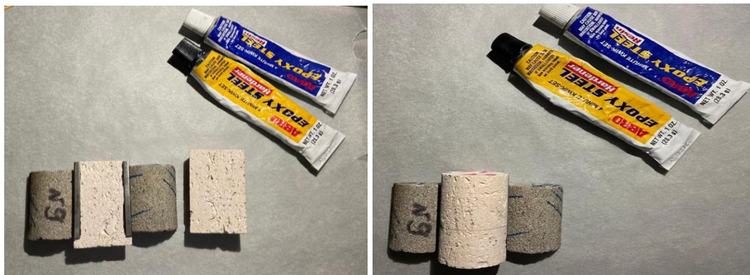
Fig. 11. Bonding of the core and the metal plate
